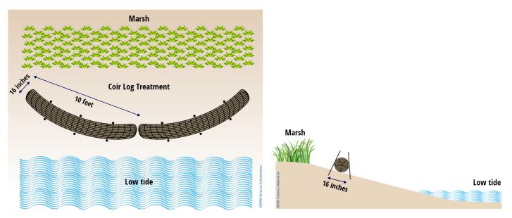
**Figure 3.14.** Overhead (left) and cross section (right) of a typical single row coir log design in the intertidal zone used for this study.
