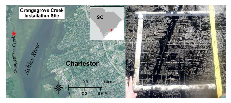
**Figure 3.11.** Living shoreline research site on Orangegrove Creek with an aerial view (left). Live oyster coverage on MWR at Orangegrove Creek in April 2019 (right) with limited recruitment and growth after 21 months.
