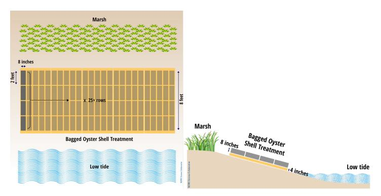
**Figure 3.3.** Overhead (left) and cross section (right) of a typical bagged oyster shell reef design with shell bags placed atop wood pallets.
