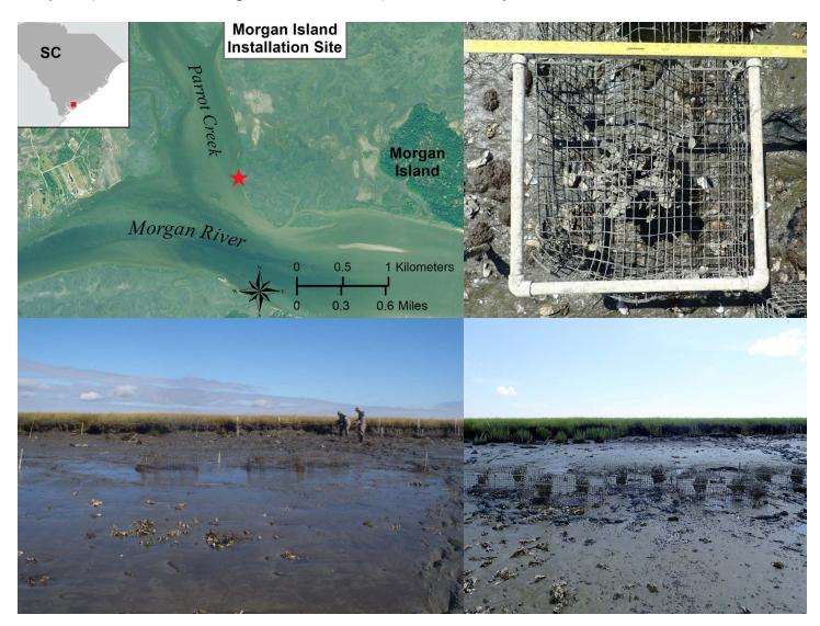
**Figure 3.12.** Aerial view of the living shoreline research site on Morgan Island Creek (upper left). Two MWR units were dislodged and relocated nearby by Hurricane Matthew (lower left) but were easily moved back into position. Live oyster coverage on MWR in August 2018 (upper and lower right).
