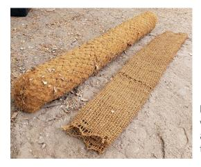
**Figure 3.13.** Coir log (10 ft length x 16 in diameter; 3 m x 41 cm) with a single-layer tube of coir netting with smaller openings and additional netting placed under the coir log to reduce sinking of the log into the sediment.
