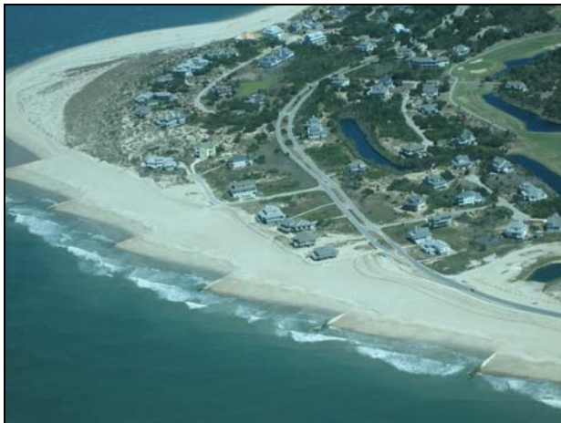
Figure 5-8: A groin series and its resultant saw-toothed shaped post construction beach (left) and a single groin (right).
