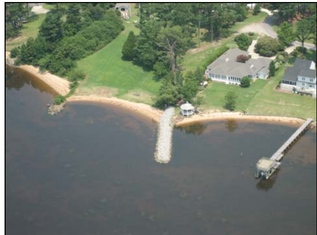
Figure 5-8: A groin series and its resultant saw-toothed shaped post construction beach (left) and a single groin (right).
