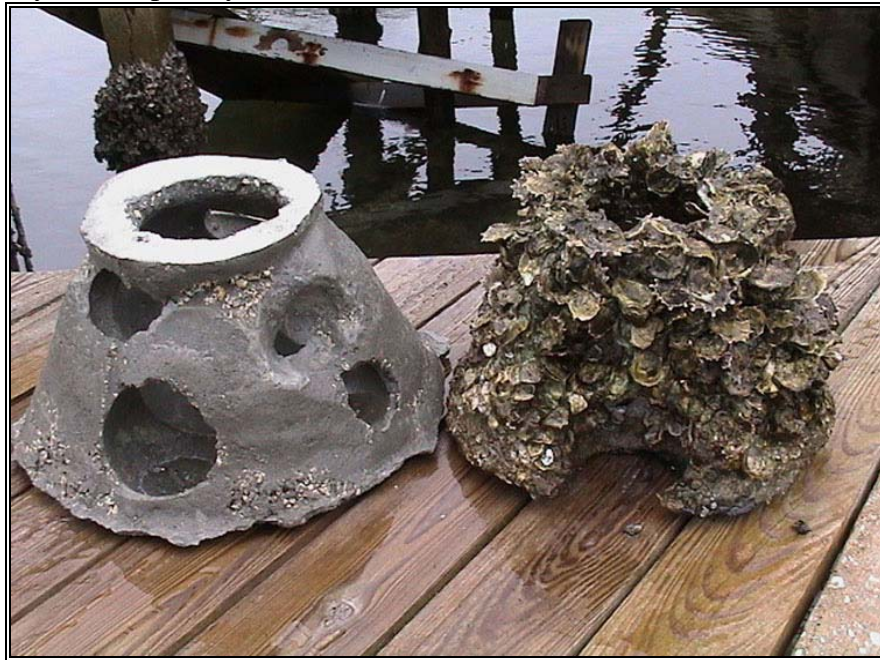
Figure 8. Oyster domes before (left) and after (right) six months placement in the water. (Photo courtesy of Tampa BayWatch)
