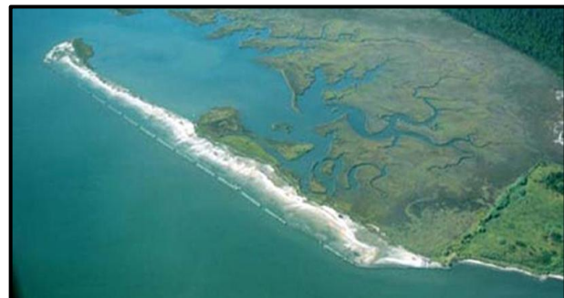
Figure 17. Wave attenuation structures used to protect and restore marsh. Bayou La Batre, AL. South Coast Engineers.
