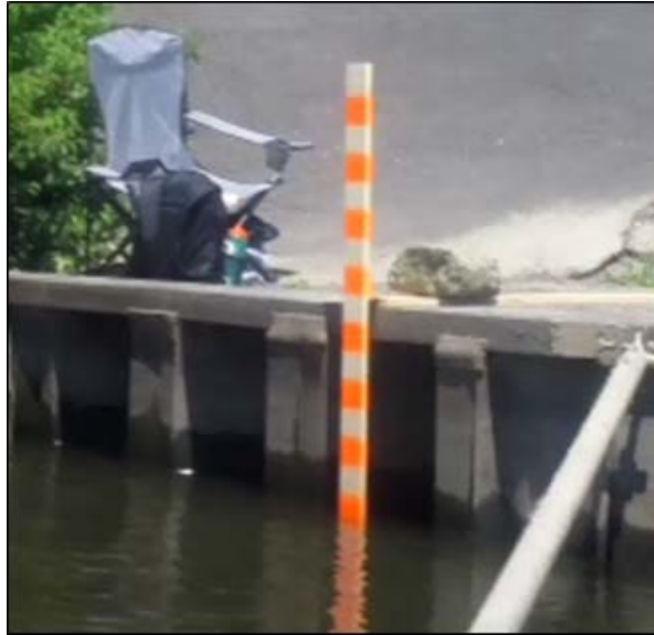
Figure 4: Visual Wake Measurement near a Bulkhead
